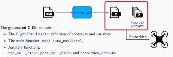
$\implies$  Compiled with the autopilot and embedded on the drone.
